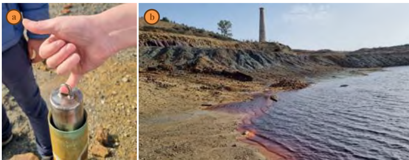
Figure 1. a) Muon borehole probe test-fitted inside an NQ-size borehole at the São Domingos pilot site. b) Stockpiles and associated highly acidic waters (pH 0) at the São Domingos pilot site in Portugal. Images: Muon Solutions.
