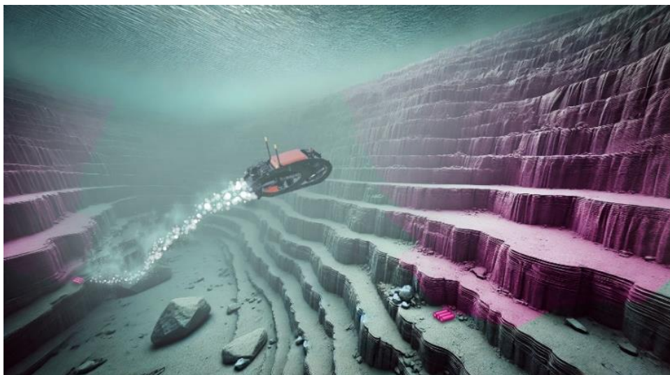
Figure 1. Concept art depicting INESC-TEC's EVA robot deploying muon detectors (pink cylinders) in a flooded open-pit environment. The regions being scanned by the detectors are coloured in pink. Image: Muon Solutions.
