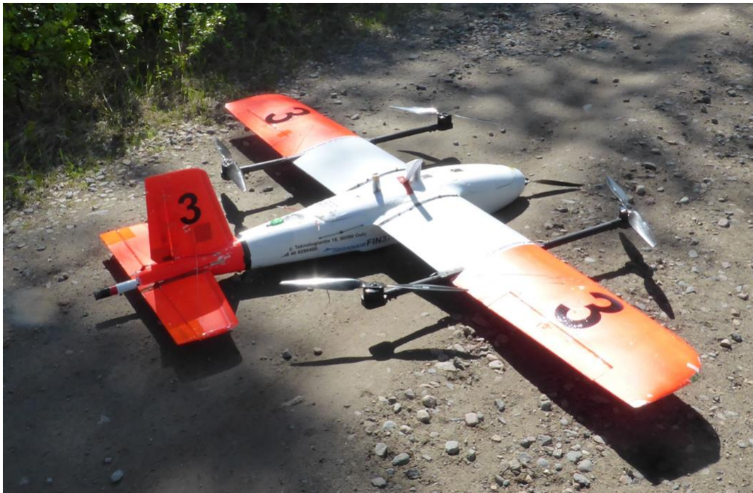
Figure 1. Coot (Nokikana) VTOL drone used in Radai's magnetic and electromagnetic surveys. A digital 3-component fluxgate magnetometer is installed inside the extended tail-pipe. The drone has electric engines and an endurance of about two hours.
